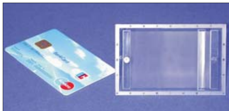
Fig 1: Chip-Design. A: Schematic representation, B: Photographical representation. L/B/H: 88 mm x 56.5 mm x 2mm; 300 parallel microchannels: 64 mm x 50 \mu\text{m} x 50 \mu\text{m} ; separation length 60 mm. Buffer reservoirs: 46.5 mm x 6 mm; IEF-cavity: 47 mm x 6 mm x 1.5 mm; Transfer gap: 47 mm x 100 \mu\text{m} x 200 \mu\text{m} ; (reduction of width in 200–250 \mu\text{m} depth from 100 \mu\text{m} to 50 \mu\text{m} ).
